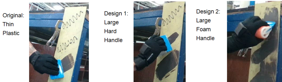
Figure 10: Original spreader, followed by two prototypes aiming to improve the design
