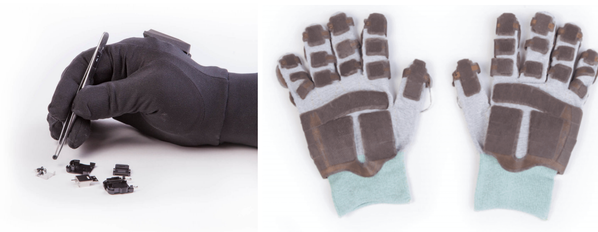
Figure 2. (a) The PPS TactileGlove being used for a task requiring good hand dexterity. (b) The inside of the TactileGlove showing the capacitive sensors.
