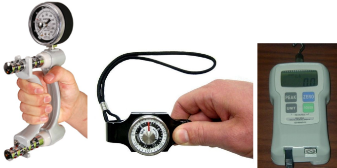
Figure 1 Traditional methods of hand force measurement (a): hand dynamometer, (b) pinch gauge, (c) push/pull force gauges.
