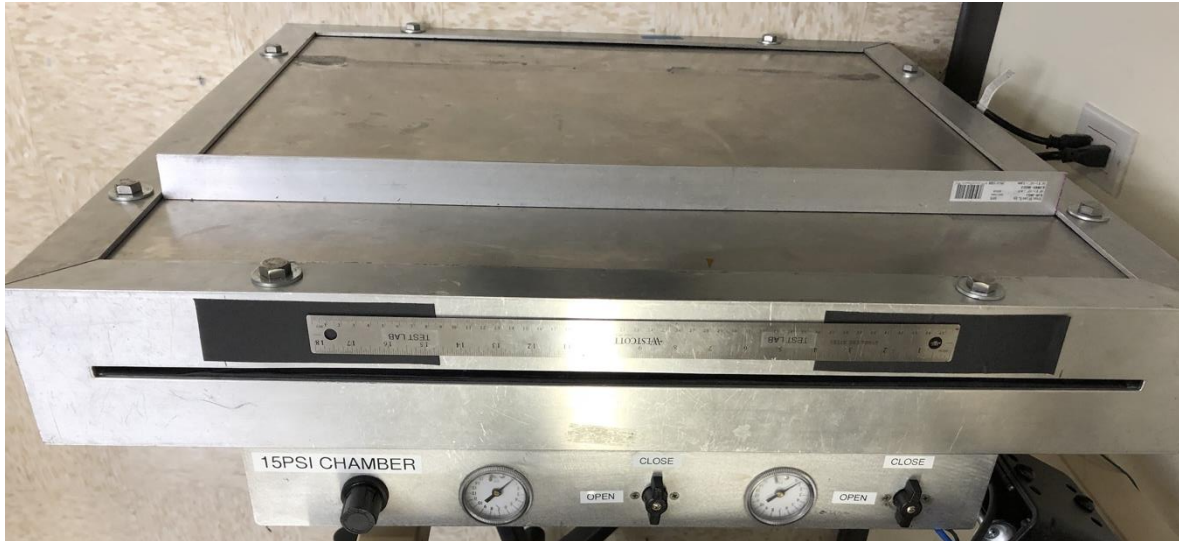
Figure 4 - Large Area Calibration Chamber
